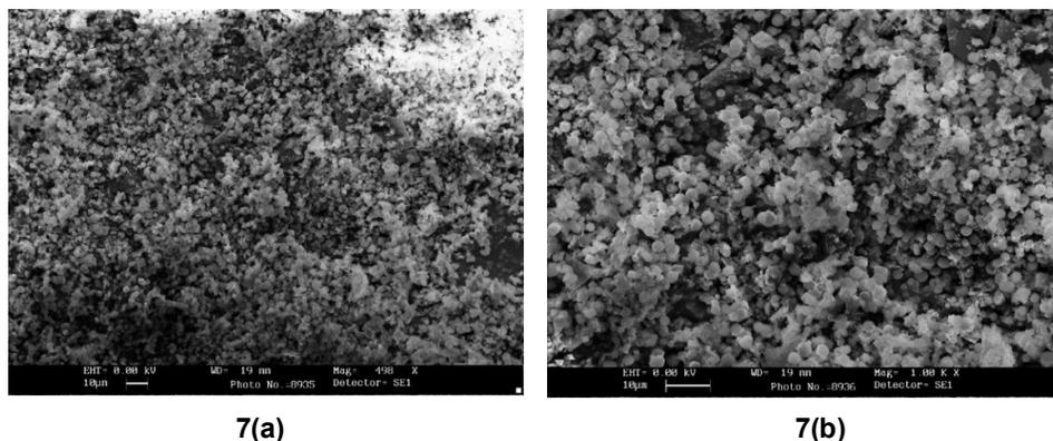
**Fig. 7:** SEM images of nanocomposite copolymer of APy and DMA at (a) 500X and (b) 1000X magnification.
