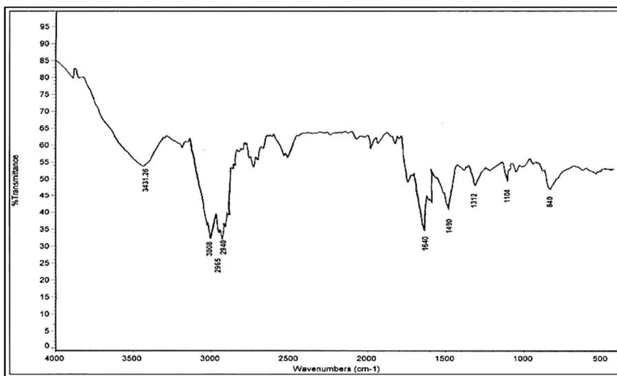
**Fig. 3:** FTIR of homopolymer of 2,3-Dimethyl aniline (DMA).
