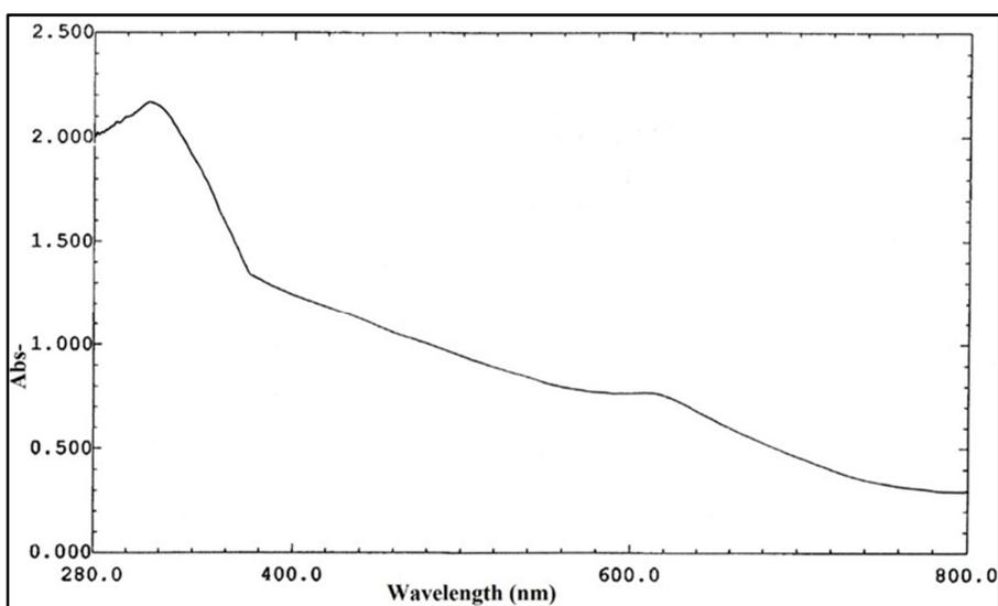
**Fig. 1:** UV-Vis absorption spectra of copolymer nanocomposite of 1-(2-Aminophenyl) pyrrole (APy) and 2,3-Dimethyl aniline (DMA).
