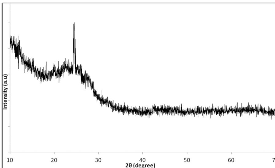
**Fig. 6:** XRD spectrum of nanocomposite of copolymer of APy and DMA.
