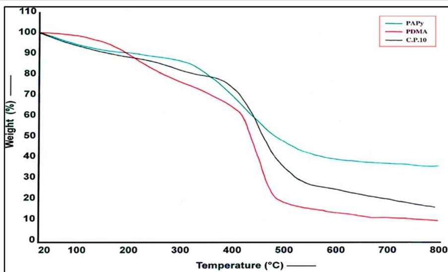
**Fig. 5:** TGA curves of APy, DMA and nanocomposite of copolymer of APy and DMA.
