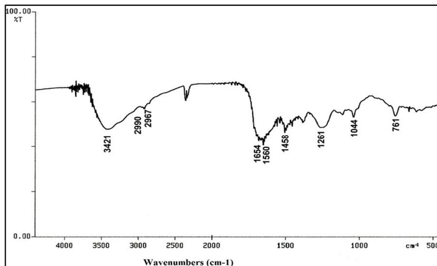
**Fig. 4:** FTIR of copolymer of 1-(2-Aminophenyl) pyrrole (APy) and 2,3-Dimethyl aniline (DMA).
