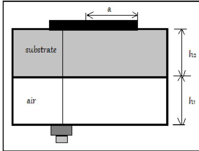
Fig. 1 : CPA with air gap.
