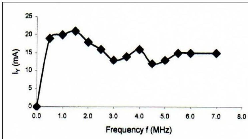
**Fig. 5:** The frequency dependent current component  $I_y$  in 10% Pr-doped  $Y_{123}$ ,  $V_x = 2V$ ,  $H_z = 6KG$ .
