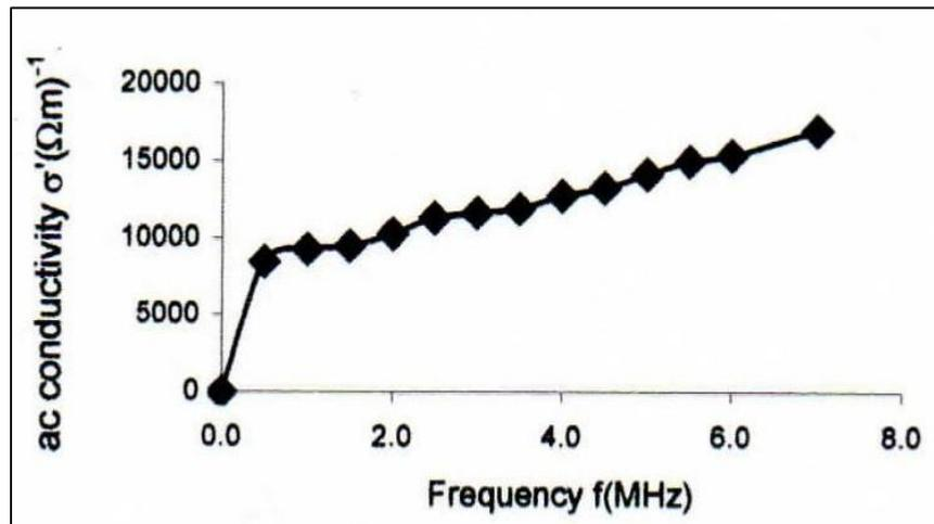
**Fig. 1:** The RF stimulated ac conductivity in 10% Pr-doped HTS  $Y_{123}$ .
