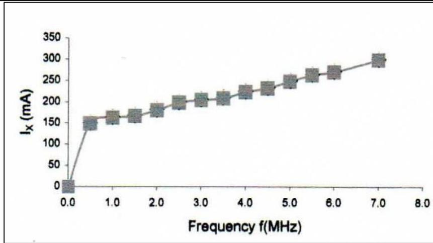
**Fig. 4:** The frequency dependent current component  $I_x$  in 10% Pr-doped  $Y_{123}$ ,  $V_x = 2V$ ,  $H_z = 6KG$ .
