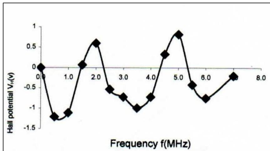
**Fig. 3:** The RF stimulated Hall voltage in 10% Pr-doped  $Y_{123}$ ,  $V_x = 2V$ ,  $H_z = 6KG$ .
