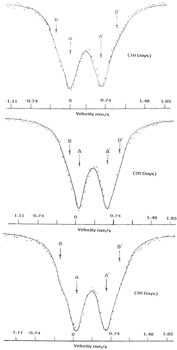
**Fig. 1:** Mössbauer Spectra(s) of Rust due to exposure of mild Steel in 1M Na<sub>2</sub>SO<sub>4</sub> solution.
