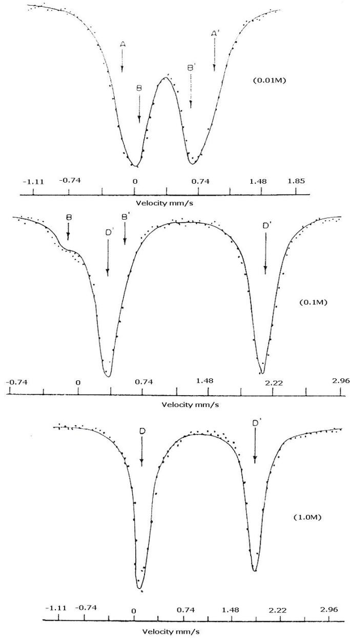
**Fig. 2(b):** Mössbauer Spectra(s) of rust due to Exposure of Mild Steel in 1M Na<sub>2</sub>SO<sub>4</sub> Solution containing Ascorbic Acid of different concentration (Exposure time 60 days).
