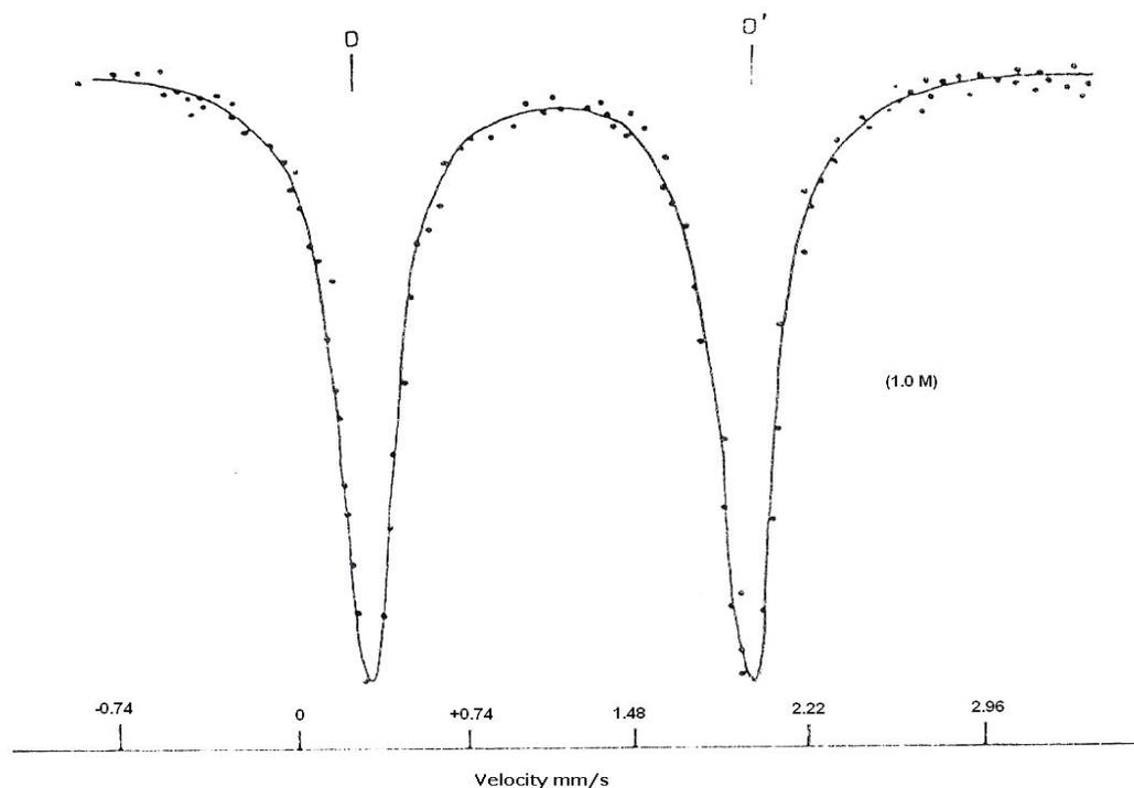
**Fig. 2(c)** Mössbauer Spectra(s) of rust due to Exposure of Mild Steel in 1M  $\text{Na}_2\text{SO}_4$  Solution containing Ascorbic Acid of different concentration (Exposure time 90 days).
