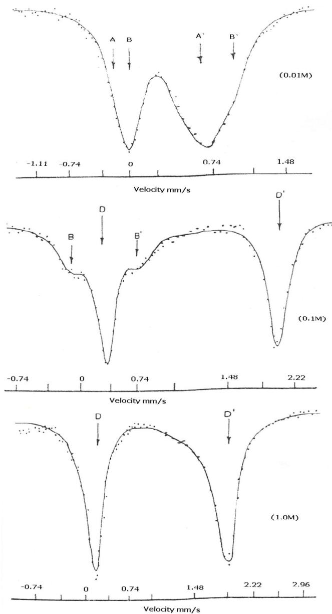
**Fig. 2(a):** Mössbauer Spectra(s) of rust due to Exposure of Mild Steel in 1M Na<sub>2</sub>SO<sub>4</sub> Solution containing Ascorbic Acid of different concentration (Exposure time 30 days).
