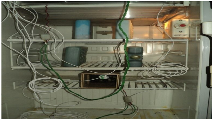
Fig. 4: Statical van with PCM, sensor and fan.
