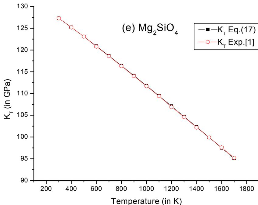
**Fig. 2:** Temperature variation of bulk modulus ( $K_T$ ) for (a) MgO, (b) NaCl, (c) KCl, (d) Al<sub>2</sub>O<sub>3</sub> and (e) Mg<sub>2</sub>SiO<sub>4</sub>.
