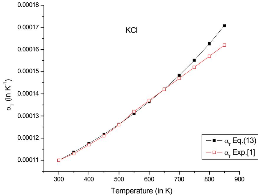
**Fig. 1(b):** Thermal expansion coefficient Vs temperature for KCl.
