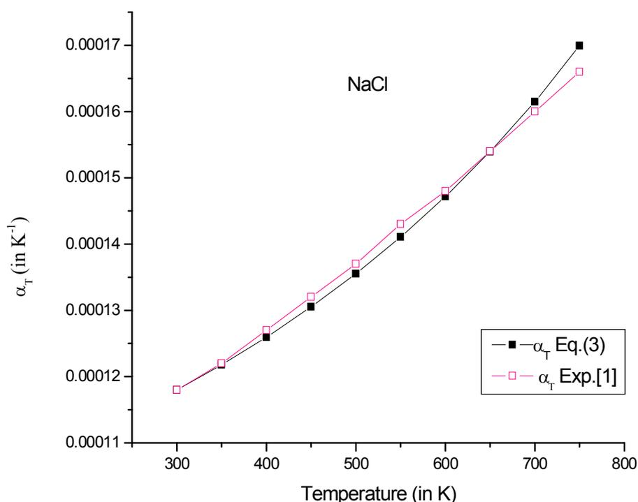
**Fig. 1(a):** Thermal expansion coefficient Vs temperature for NaCl.
